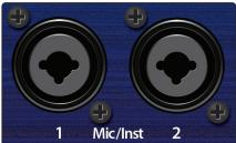
Microphone/Instrument Inputs. Both channels of the AudioBox USB96 have Mic/Instrument combo jacks. This convenient connector accepts either a 1/4-inch phone plug or an XLR plug.
